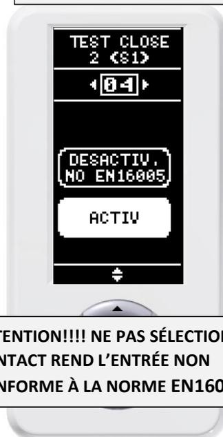
**ATTENTION!!!! NE PAS SÉLECTIONNER LE CONTACT REND L'ENTRÉE NON CONFORME À LA NORME EN16005.**
