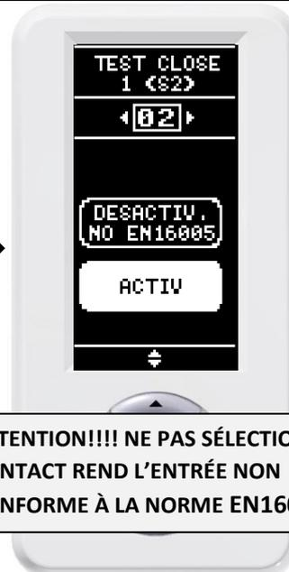
**ATTENTION!!!! NE PAS SÉLECTIONNER LE CONTACT REND L'ENTRÉE NON CONFORME À LA NORME EN16005.**
