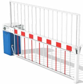
BARRIERE LEVANTE JUSQU'A 6 M AVEC HERSE HAUTE FIXE ET BASSE ARTICULEE LISSE ALUMINIUM 175 X 75 MM BARREAUX DE DIAM 20 MM
