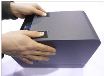
Open the Espas 20T cover fully without disconnecting the device and pushing the levers on the lid.
