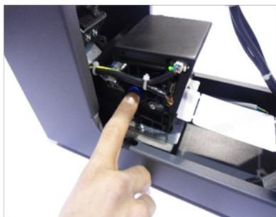
Remove any ticket from the printer pressing the blue side lever shown in the photo, the correct operation will be highlighted by a red LED on the printer itself.
