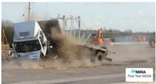
Has been successfully crash tested, in accordance with the IWA 14-1:2013 specification, as a
